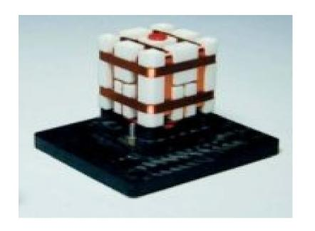
Fluxgate-Magnetometer with a resolution of at least 40 pT
