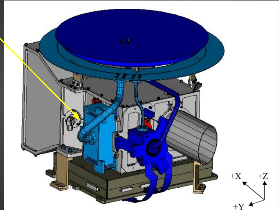
*Figure 10-1: A model of Ralph in the spacecraft coordinate system. The Ralph aperture points in the  $-X$  direction, the normal to the radiator is in the  $+Z$  direction and the SIA points in the  $+Y$  direction.*
