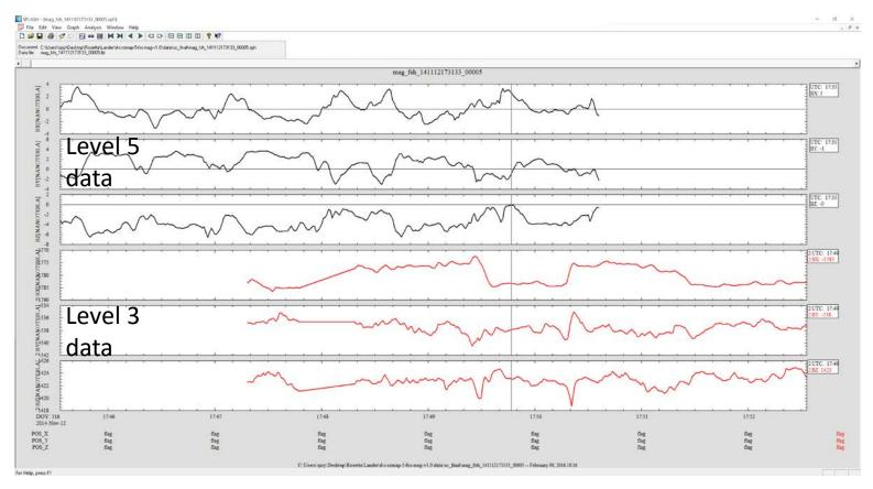
Plot generated from data file by reading label mag\_fsh\_141112173133\_00005.lbl and format file romap\_mag\_calsch.fmt (labels valid). Black traces are derived data, red traces are the preliminary data for the same time period. **Trajectory columns are all missing data flags in the data file.**
