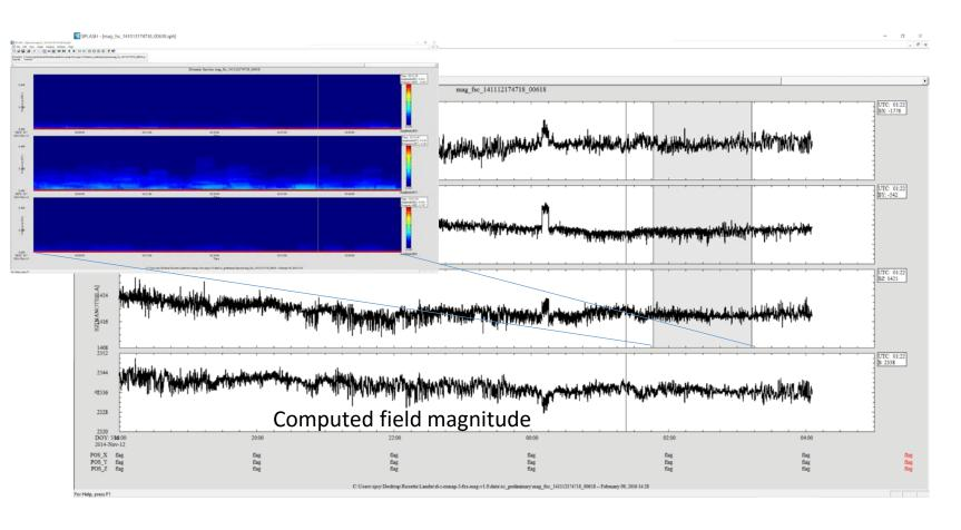
Plot generated from data file by reading label mag\_fs2\_141112174718\_00618.lbl and format file romap\_mag\_rawsc.fmt (labels valid)
