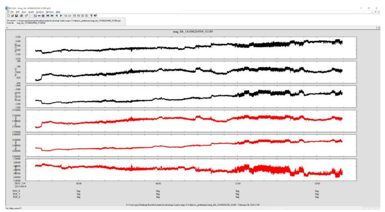
Plot generated from data file by reading label mag\_fsb\_141006204506\_01389.lbl and format file romap\_mag\_calscb.fmt (labels valid). Black traces are calibrated data, red traces are the raw data for the same time period. Trajectory columns are all missing data flags in all data files.
