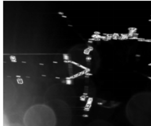
Figure 1. Left: Mounting of the LAP sensors on Rosetta at the tips of the two solid booms, as well as other RPC sensors and units. Right: Both LAP probes are visible in this image by ROLIS on Philae shortly after its separation from Rosetta, from a similar angle.
